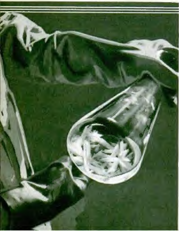
White crystals of radium bromide appear in colorless liquid during final stage of refining by Canadian Radium & Uranium Co.
